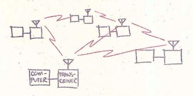
Figure 1. Computers communicate directly with neighbors and through relays with the remainder of the network.
