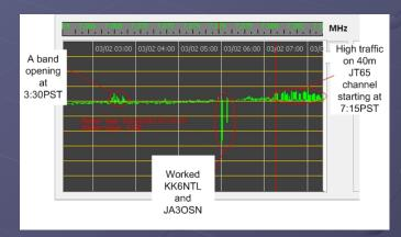
On the left: detection of solar flare and a rare 40m 3AM PST band opening.
