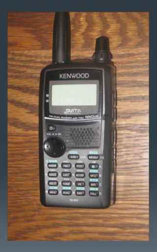
Portable radio with built in TNC.
