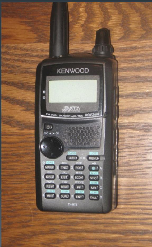
Portable radio with built in TNC.
